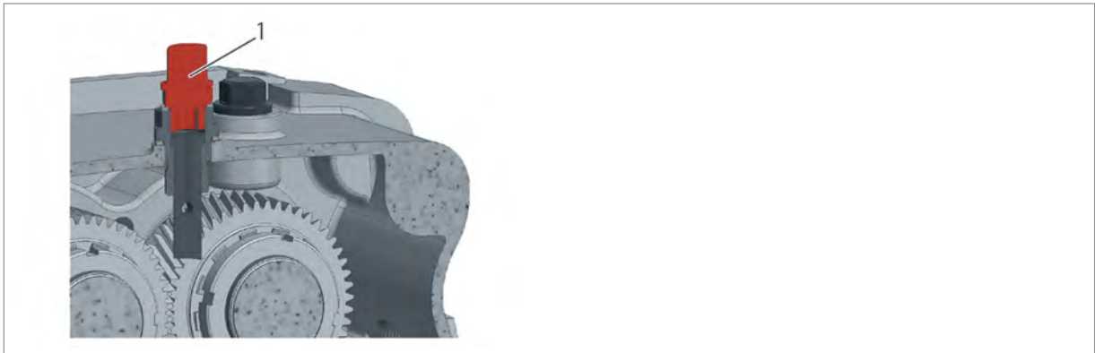
Fig. 10: Ventilation filter on the bearing casing
