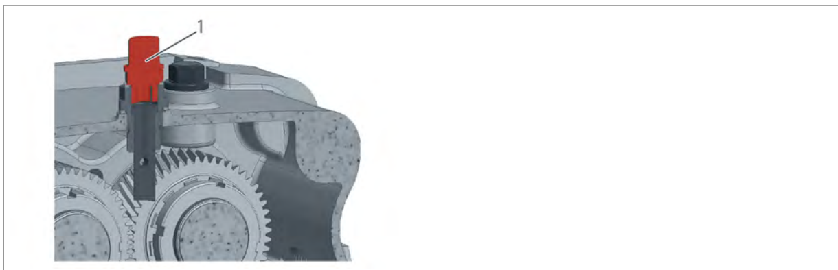
Fig. 9: Ventilation filter on the bearing casing
