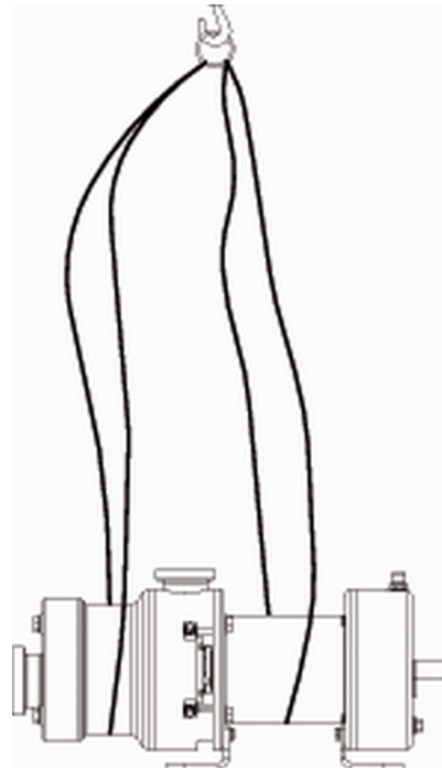
Fig. 5: Fastening the lifting tackle to the pump
