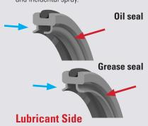
Sealing Lip firmly grips the shaft and wears away after prolonged use maintaining the shaft integrity. Grooving becomes virtually non-existent.
