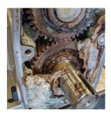
Water and debris enter a gear case past old style shaft seals through high pressure washing causing oil break down and rusting of gears and bearings
