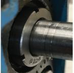
Shaft-grooving can develop overtime from traditional spring loaded lip seals causing a pathway for contaminants to enter and allow oil to escape which results in costly and time-consuming shaft and bearing replacement
