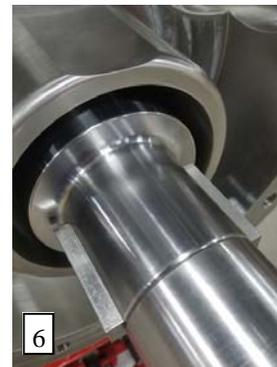
**BODY REMOVAL PROCESS- FLUID HEAD DISASSEMBLY**
