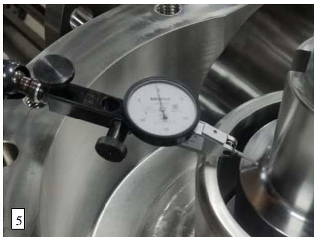
**GERACASE ASSEMBLY - SHAFT INSTALLATION**
