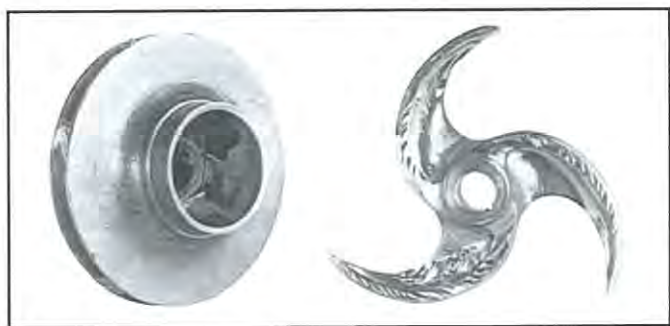
FIGURE 1 — Compare the open impeller after 3 months, and the closed design after 3 full years of pumping the same slurry at identical speed, capacity and head. Open impeller, badly worn on vane faces, had lost so much capacity it had to be replaced.
