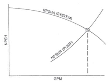
To satisfy the suction requirements, the pump must be operated at a capacity less than the intersection point of the NPSHA and NPSHR. At operation beyond this point, one can expect a cavitating state to exist.
