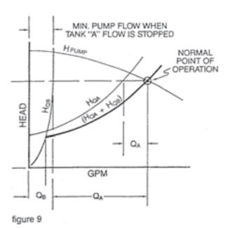
A graphical analysis (figure 9) can be made to illustrate what develops when a by-pass orifice is introduced.
