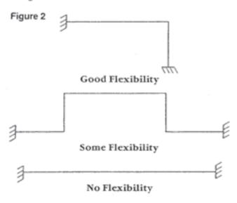
Bending stresses due to thermal expansion are not significantly affected by increasing pipe wall thickness. Rather, increasing wall thickness has an even more undesirable effect in that the reacting forces and movements are increased in a direct ratio.
