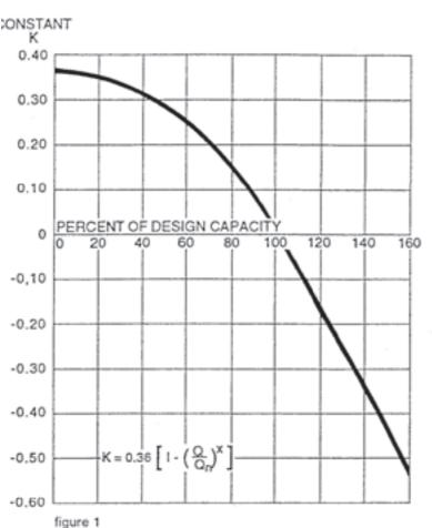
The graph indicates that, on both sides of the best efficiency point this equilibrium of volute pressure - a highly significant pressure differential develops as the point of operation moves in either direction away from the pump's design point.
