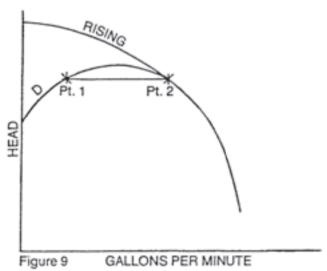
The effect of this can be a "hunting action" between the two points, causing variations in capacity and pressure. The beginning of the pressure variation lies in the fact that, at some time, the pressure in the discharge line is higher than that developed in the pump and a movement to reverse flow occurs.
