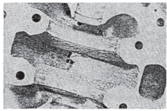
Figure 3: Corrosion Erosion
