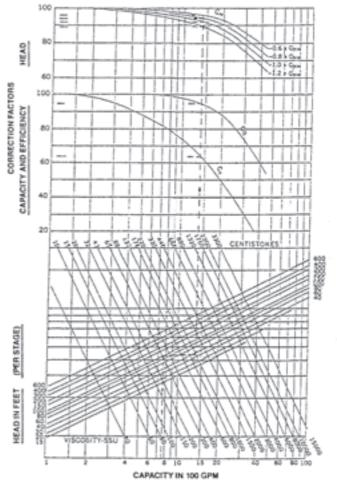
FOUR POINT DETERMINATION PERFORMANCE CORRECTION CHART FOR VISCOUS LIQUIDS
